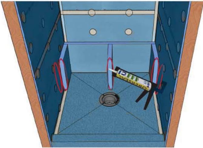
f) To adhere front 2" board , repeat step c.
