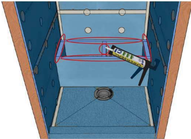
h) To adhere the top 2" board , repeat step c.
