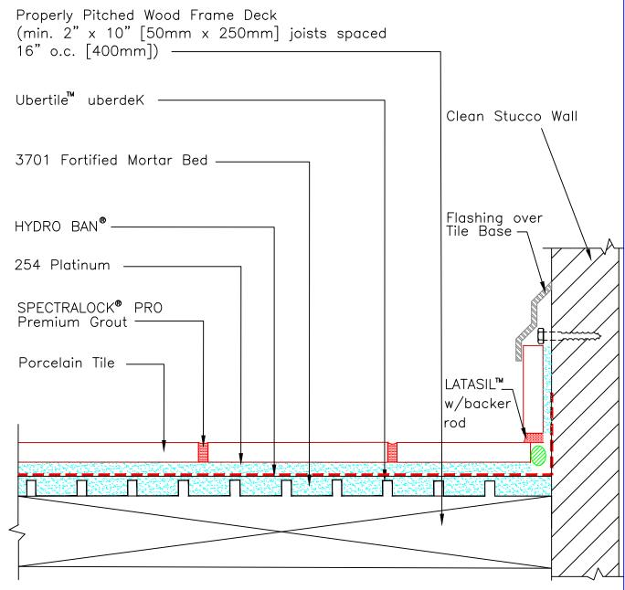
NOTE: This method is not for use over living space. Minimum tile size of  $8" \times 8"$  (200mm x 200mm) and maximum tile size of  $24" \times 24"$  (600mm x 600mm)
