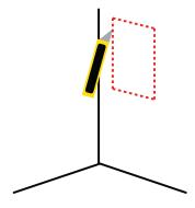
If necessary, remove screws/washers in the cut path. Carefully cut the UberBoard wall panel and remove the cut-out.
