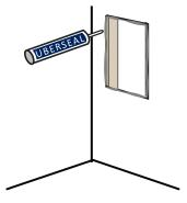
Apply Uberseal to the exposed foam edge of the UberBoard wall panel arund the entire perimeter of the cutout.
