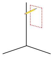
Mark onto the 1/2" UberBoard Wall Panel where your niche is to be installed. The markings must line up to the centre of the 16" O.C. studwork.
