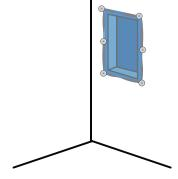
Use a minimum of 6 Ubertile Screws and Washers to fasten the niche to the wall.
