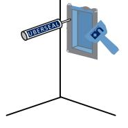
Apply Uberseal to the entire Niche perimeter. Ensure screws are fully covered. While the Uberseal is wet, smooth it flat with the spreader so there is a minumum of 1" overlap of sealant onto both the niche and Uberboard surfaces.
