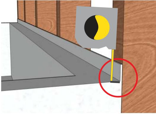
1. Measure the dimension of the Bathtub Vertical Flange.
