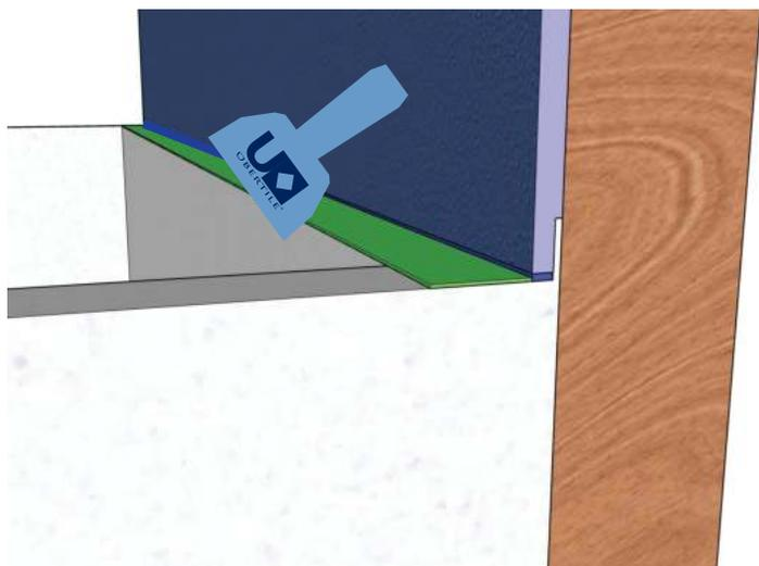
5. With the Uberseal™ still wet, spread the Uberseal™ flat, ensuring not to spread Uberseal™ onto the finished surface of the Bathtub; The painters tape should protect the finished surface of the Bathtub.
