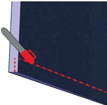
2. On the backside of the Uberboard™ panel mark the dimensions of the Bathtub Vertical Flange.
