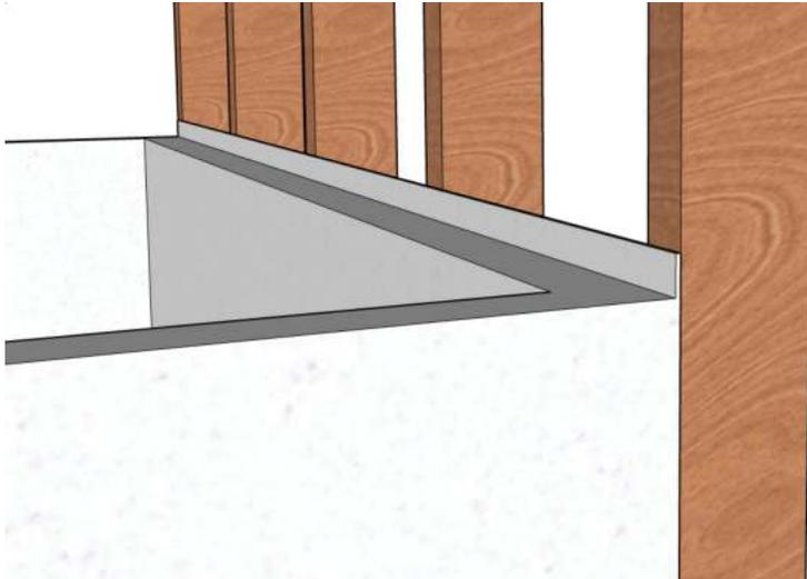
1. A Bathtub used as a “Tub/Shower” MUST have a vertical flange which extends upwards a minimum 25mm (1”) upwards from the Bathtub deck.
