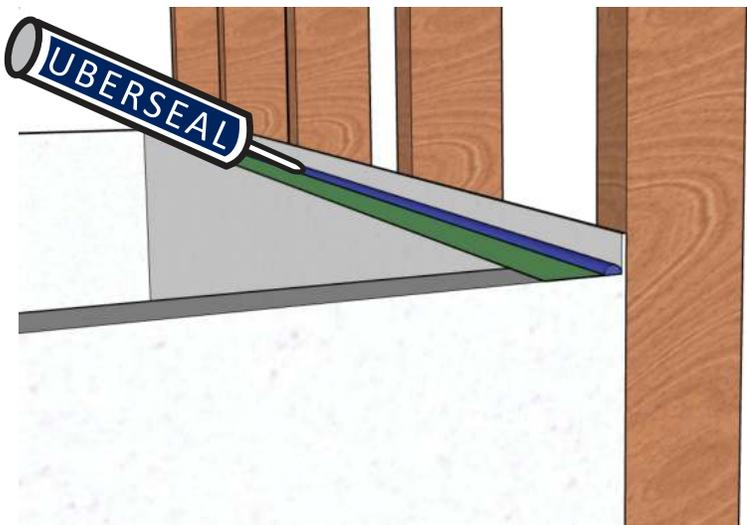
3. Apply a generous bead of Uberseal™ onto the surface of the Bathtub where the 1/2” Uberboard™ panel will be installed.
