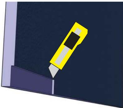
3. Use a Utility Knife (or a table saw if you want to be fancy) to cut the backside of the Uberboard™ panel, leaving a groove which will fit / contour to the shape of the Bathtub Vertical Flange.
