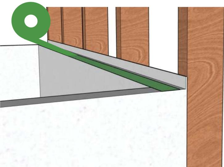
2. Apply painter's tape onto the bathtub surface, setback 12.5mm (1/2”) from the Bathtub's vertical flange.
