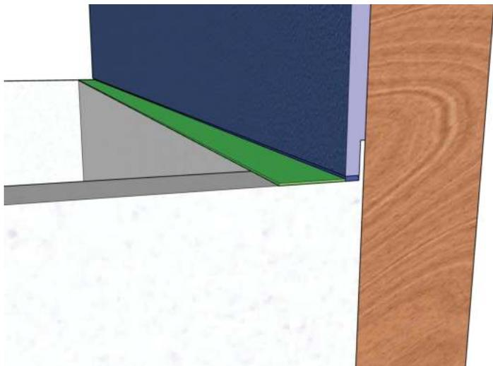
4. With the Uberseal™ still wet, place the Uberboard™ panel into the Uberseal™.
