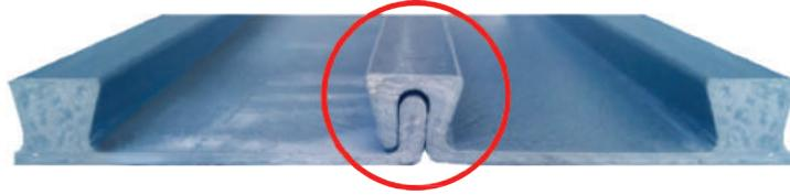
Tip: Use a rubber mallet to ensure the tongue & groove are fully clipped together. Not fully joining together the boards may result in the tiles being uneven or detaching from
