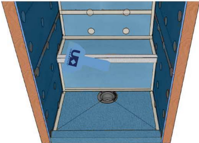
n) Embed / smoothout the fibremesh tape by tooling into the fresh modified tiling thinset .
